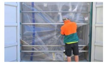
**Figure 4.** Container lined with single-use polyethylene used to transport pipe compound in bulk from the manufacturer to the pipe manufacturer.
