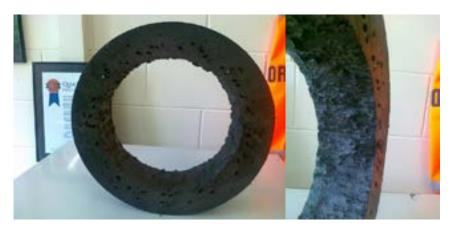
Figure 1. Effects of excessive moisture in pipe compound on PE pipe: voids in the pipe wall (left) and rough surface of inner pipe wall (right).
