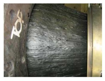
Figure 2. Excessive moisture in the pipe compound affects the quality of the finished pipe, including the appearance of the outer surface of the pipe wall. Picture shows moisture affected pipe surface during pipe manufacturing between the extruder die and sizing calibrator.
